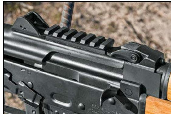
A strip of Picatinny rail mounted forward of the rear sight allows for use of micro red-dot optics.
