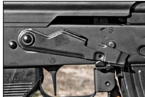
The safety has a modified cutout that can engage the charging handle and lock open the action.
