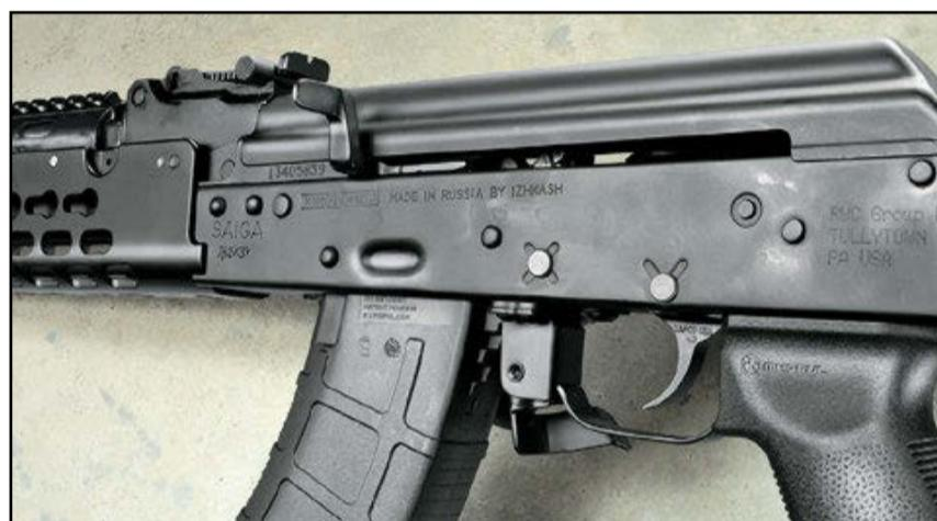
The left-side charging handle makes it possible to charge the rifle without removing the shooting hand from the rifle's pistol grip.
