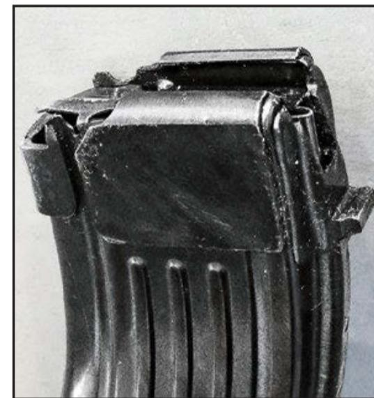
The Type-81 employs a proprietary magazine with an integrated bolt-hold-open system.
