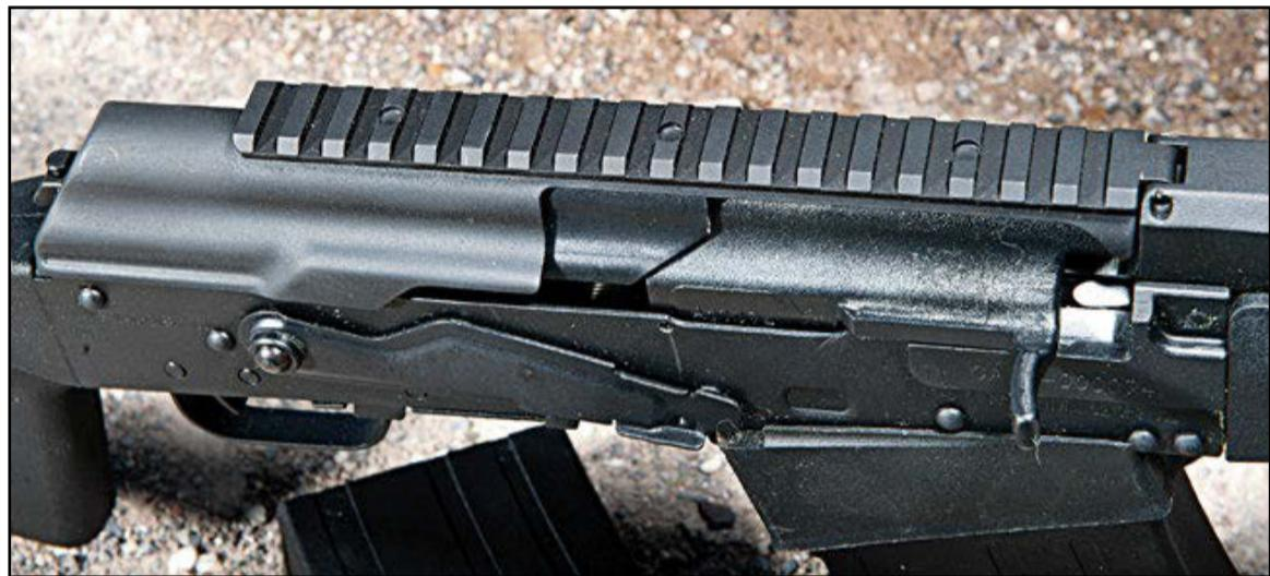
The hinged top cover of the shotgun featured a Picatinny rail anchored to the gas block portion.
