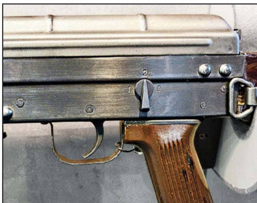
Unlike the large dustcover-style safety of the AK, the Type-81's safety selector is a smaller lever located on the left side of the receiver.
