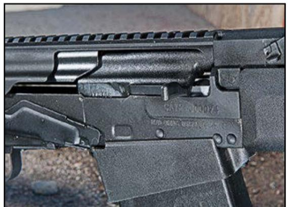
Bolt manipulation is the same as any basic AK-configured weapon. The mag funnel facilitated straight insertion with no need to rock the mags.
