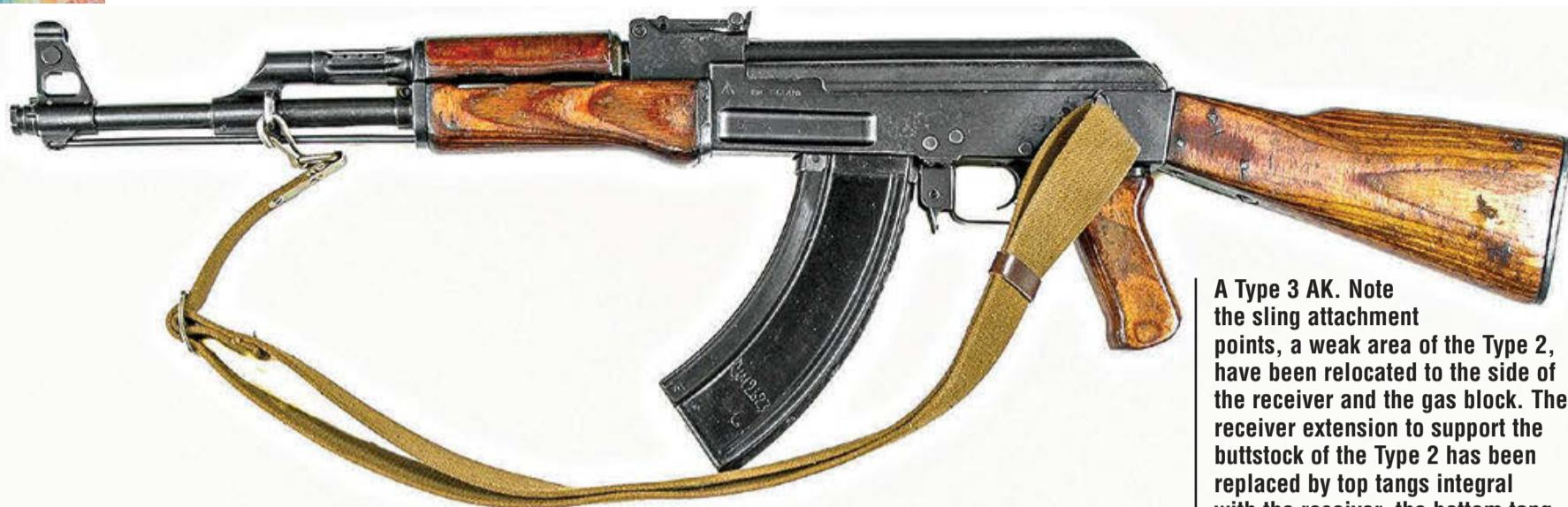
made from a single piece of wood that was attached to the receiver by a machine screw that extended vertically through the center of the grip into the receiver. The threaded boss that accommodated the grip screw was a separate machined piece, secured to the receiver under the rear trigger-guard tab with two rivets.
