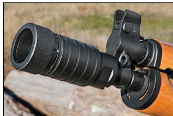
Author fitted out the threaded muzzle with a new four-piece flash suppressor/muzzle brake unit.
