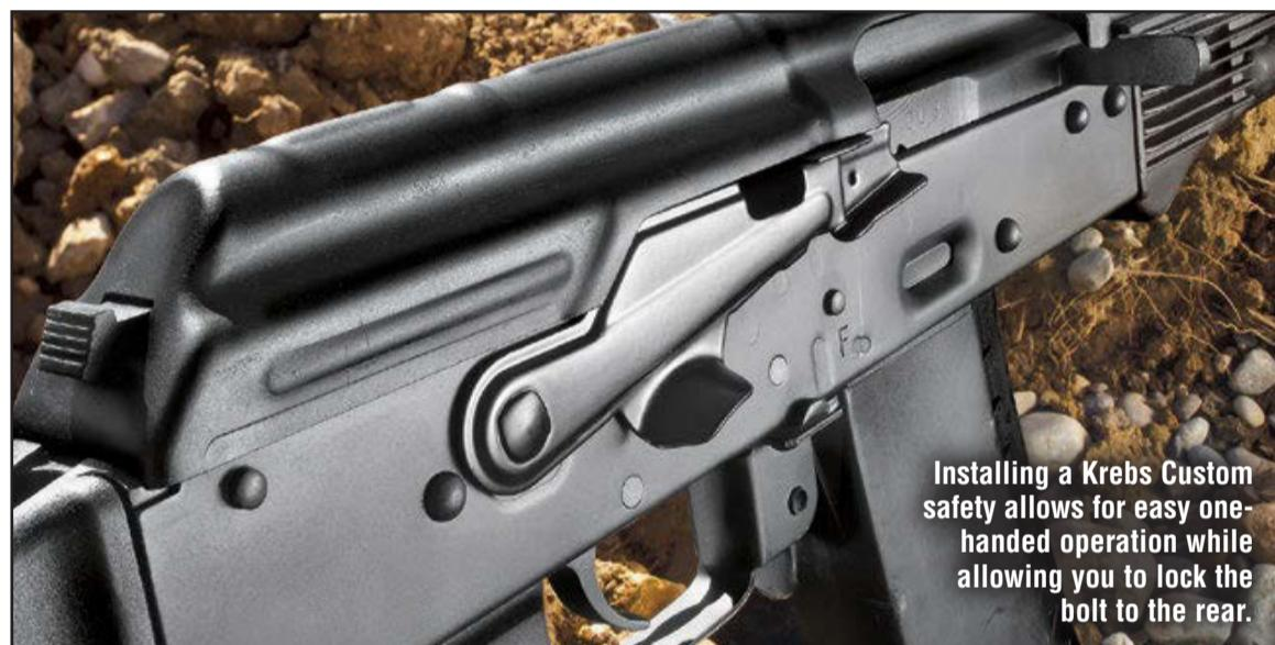
Installing a Krebs Custom safety allows for easy one-handed operation while allowing you to lock the bolt to the rear.
