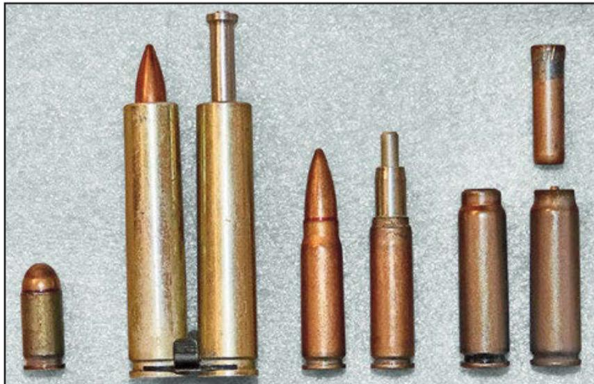
Ammo for Soviet spec-ops pistols, L to R: 9x18mm Makarov, 7.62x63mm PZ (complete round and fired case with piston extending out of the mouth), 7.62x37mm SP-3 (complete round and fired case with extended 2-piece piston), and 7.62x40mm SP-4 (complete round, fired case and fired bullet).
