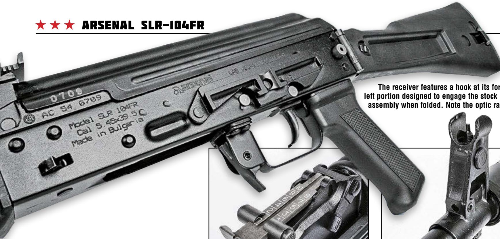
The receiver features a hook at its forward left portion designed to engage the stock assembly when folded. Note the optic rail.
