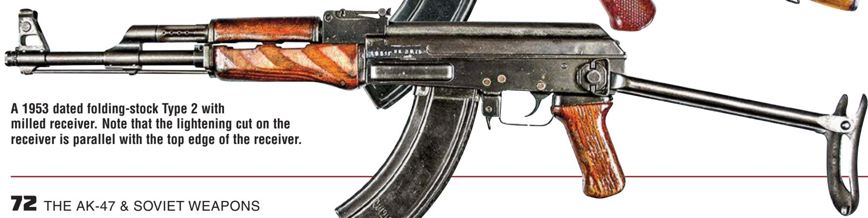
A 1953 dated folding-stock Type 2 with milled receiver. Note that the lightening cut on the receiver is parallel with the top edge of the receiver.
