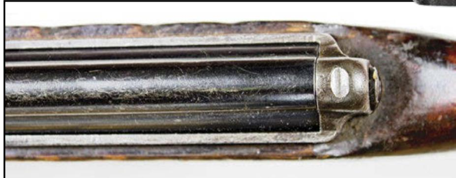
The machined recess on this early SVT is used to secure the SVT scope mount.
