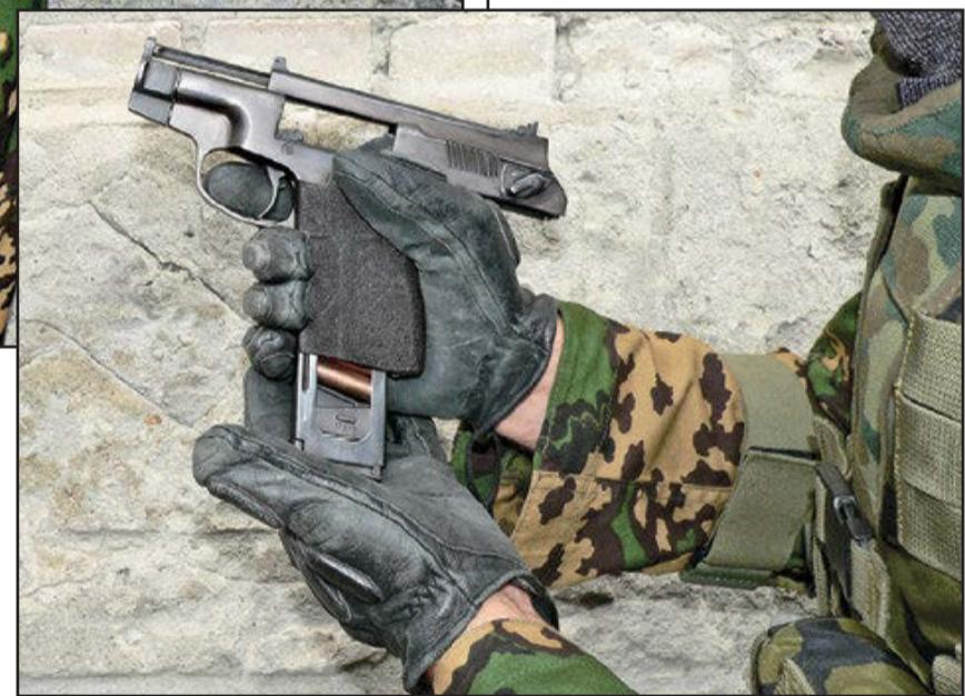
weapon that could be disguised as something that looks completely safe and fire poison-tipped bullets without any noise or flash. To achieve the latter effect, Stechkin employed the rather old principle of capturing hot powder gases (the prime source of the sound and flash during the discharge) within the confined space of the specially designed cartridge case.
