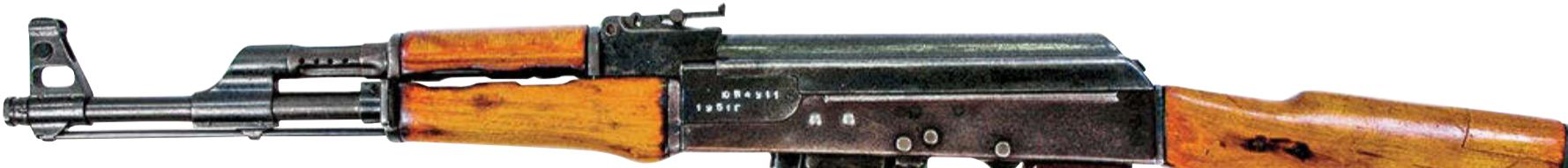
A 1951 dated Type 1 AK rifle with a stamped sheet metal receiver. The Type 1 was produced from 1949 until 1951, when it was replaced by the milled receiver Type 2.
