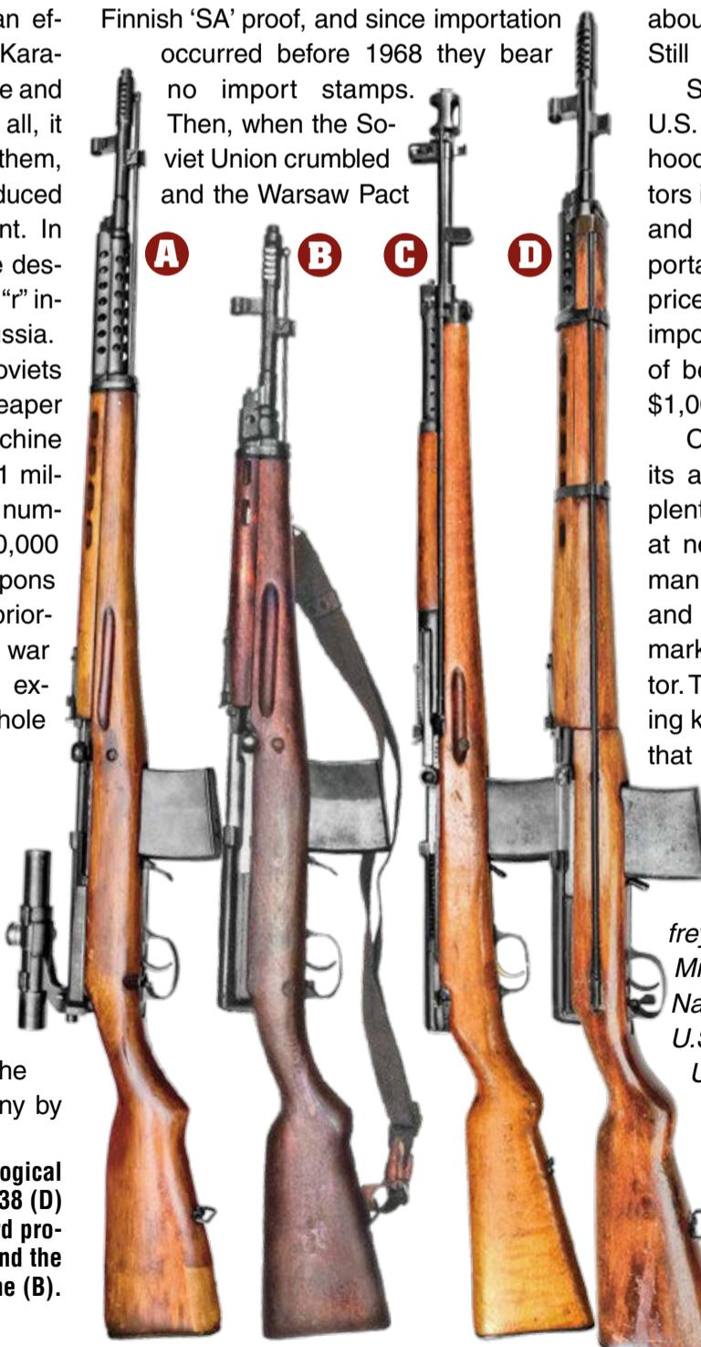
**Tokarev development in chronological order:** the select-fire AVS-36 (C), SVT-38 (D) with right-sided cleaning rod, standard production SNT-40 with PU scope (A), and the rarely encountered SKT-40 Carbine (B).
