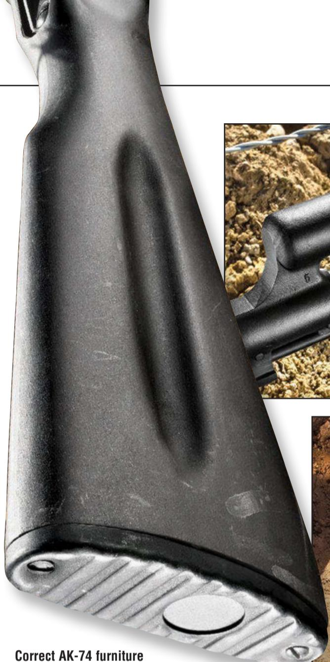
Correct AK-74 furniture provides the user with an easy to access cleaning kit door with a ribbed steel buttplate.
