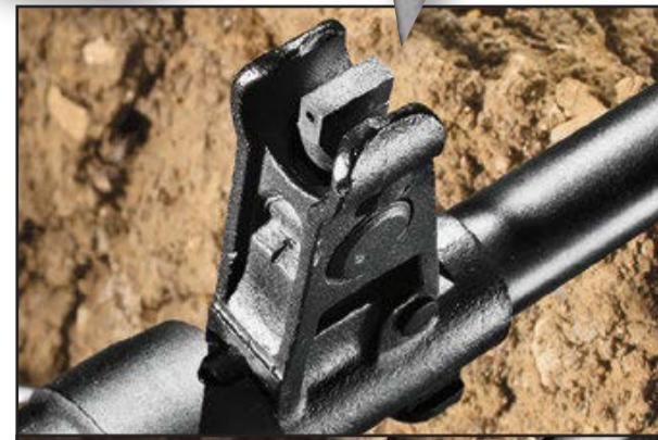
Upgrading sights to a tritium front and ghost ring rear allows for use in failing and low light.
