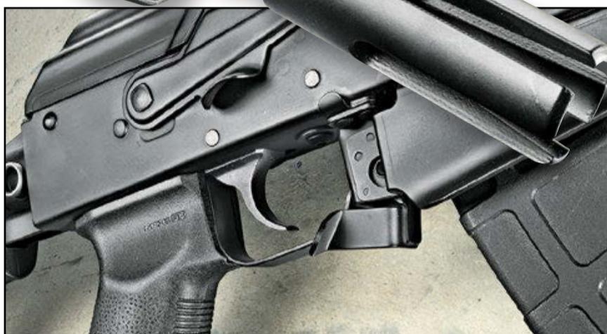
The Krebs-modified TAPCO trigger set provides a smooth, six-pound trigger pull and the rifle has a Krebs Mk VI enhanced safety.
