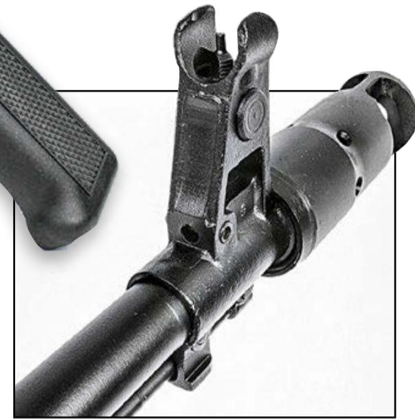
The post front sight, elevation and windage adjustable, is protected by dual steel wings that are designed to protect it from impact.
