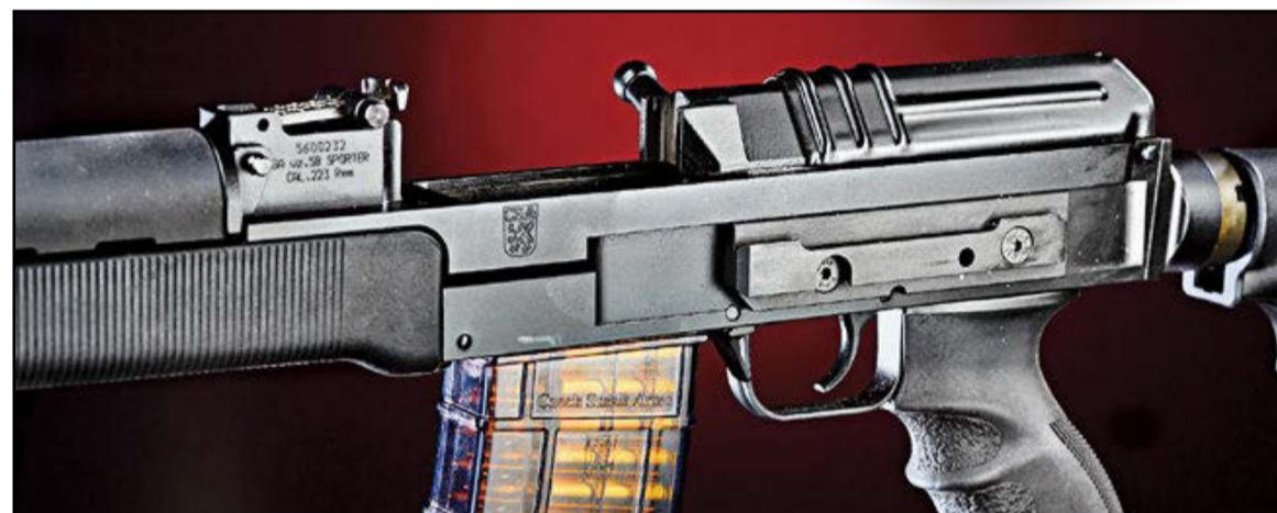
The CzechPoint vz. 58 Tactical 556 features an optics rail mounted on the left side of the receiver, allowing the supplemental use of optics in addition to the iron sights.
