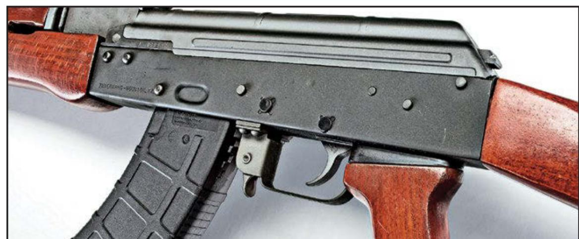
Construction (rivets, etc.) were well-done and featured an excellent parkerized finish.
