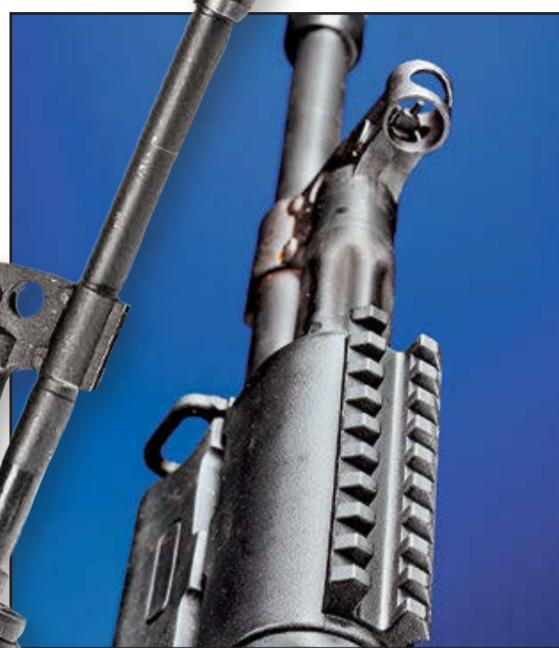
The M10-762's gas block (at left) features a modern 90-degree angle. Note integral Picatinny rail in the upper handguard (above).
