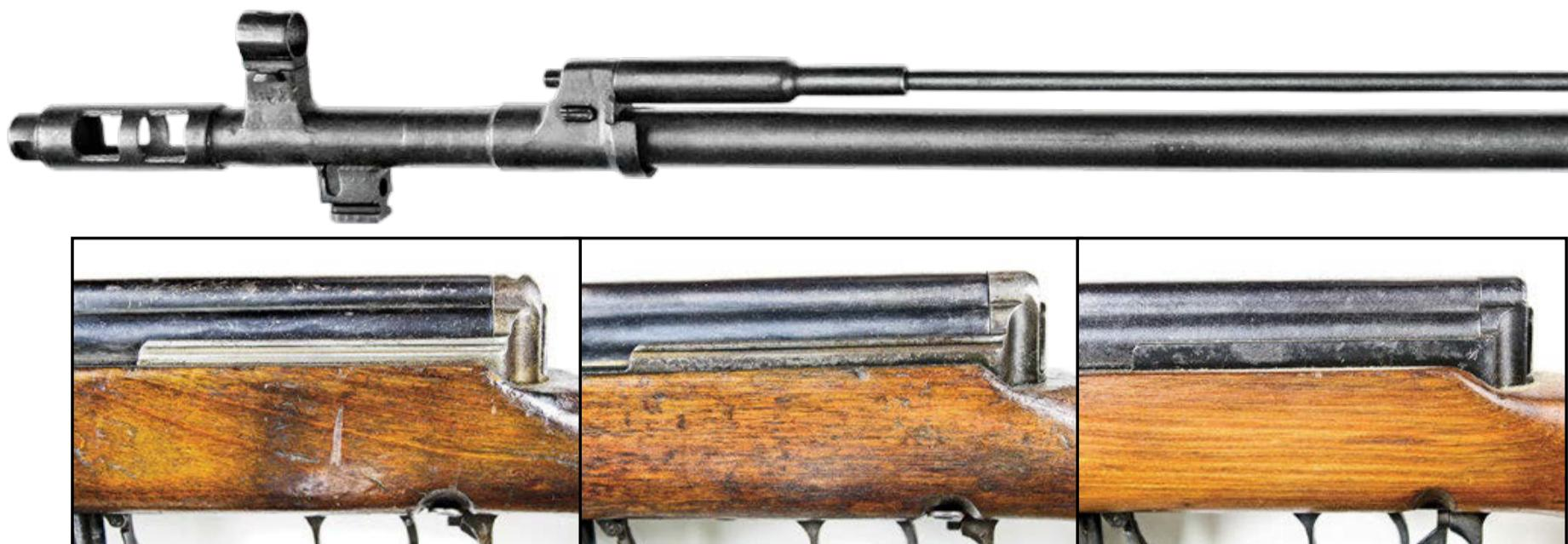
An early gun with grooves and machined recess (above, left), a later model with grooves (above, center) and an even later receiver (above, right).
