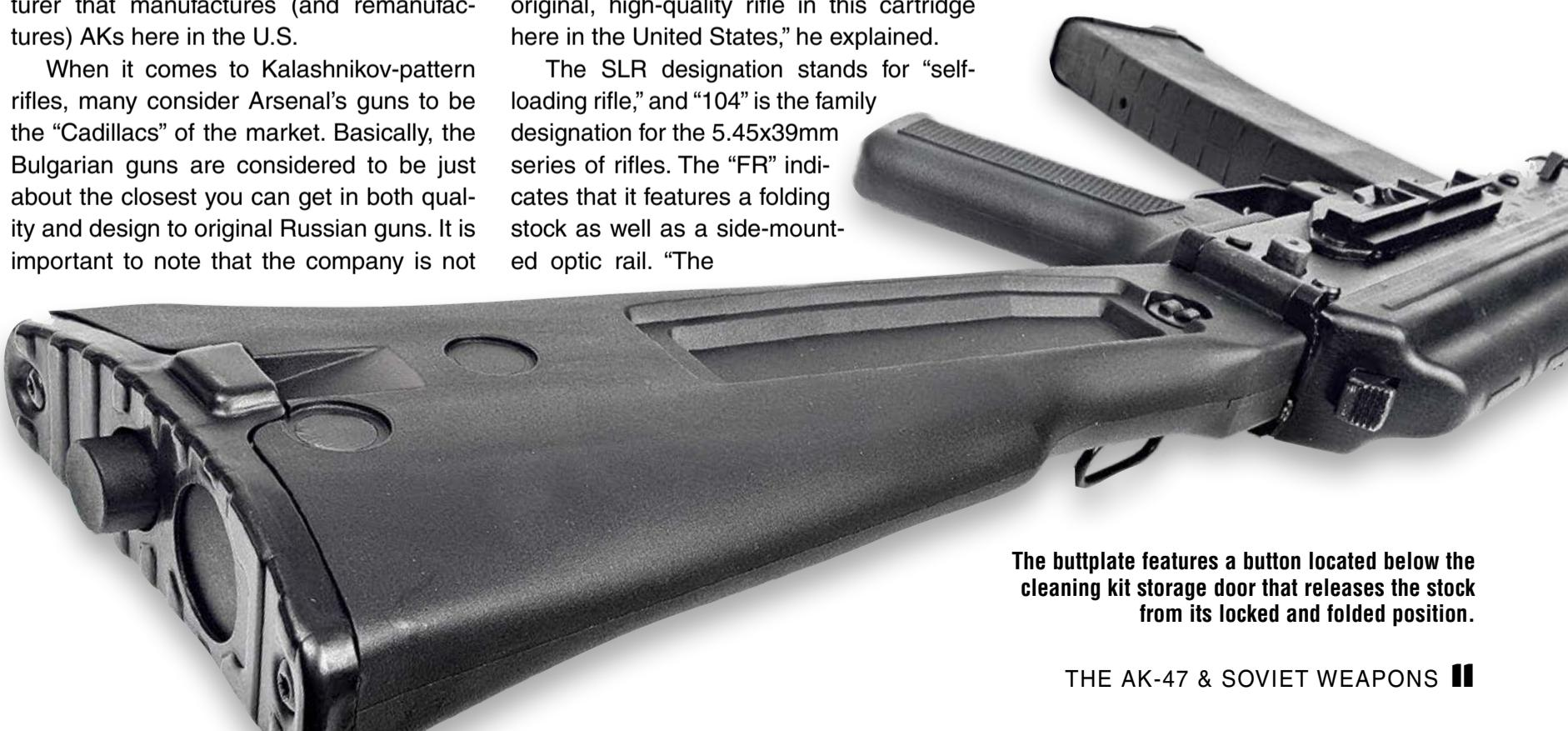
The buttplate features a button located below the cleaning kit storage door that releases the stock from its locked and folded position.
