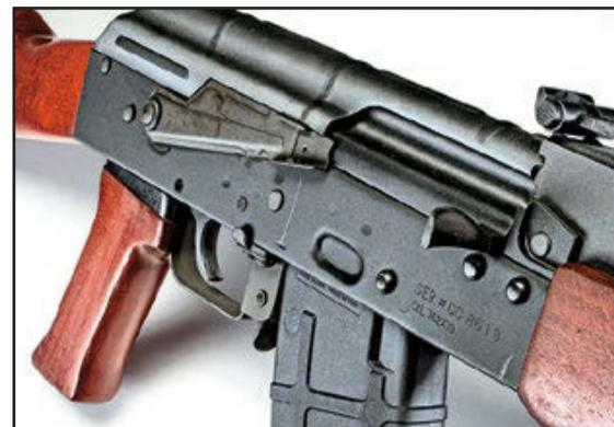
Right-side controls are standard: cocking handle, ejection port, and safety.
