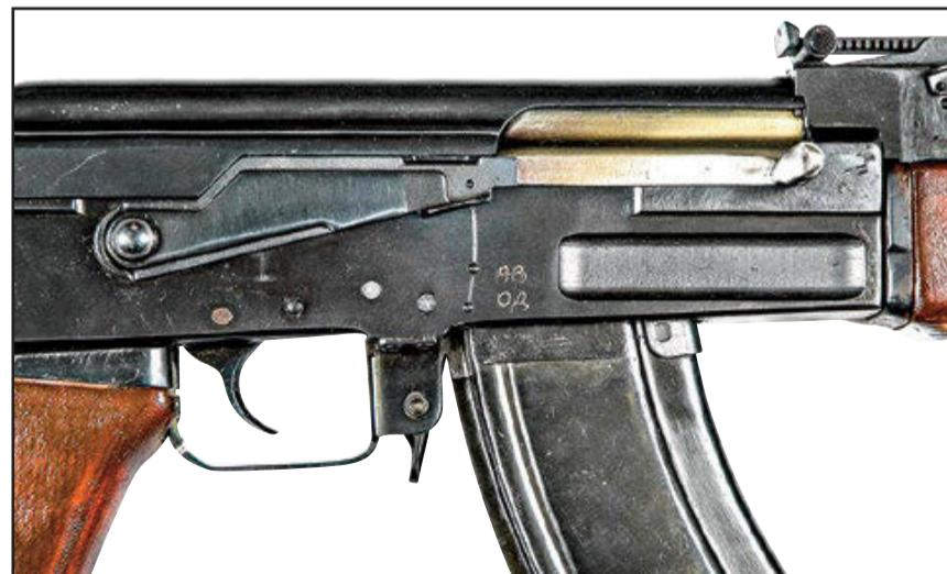
View of a Type 2 receiver's right side. The selector position markings have been hand-inscribed and the selector lever detents are round. Many Type 2 receivers lack selector position markings. The receiver has several "ledges," one below the cocking handle, the other behind the selector lever supporting the top cover.
