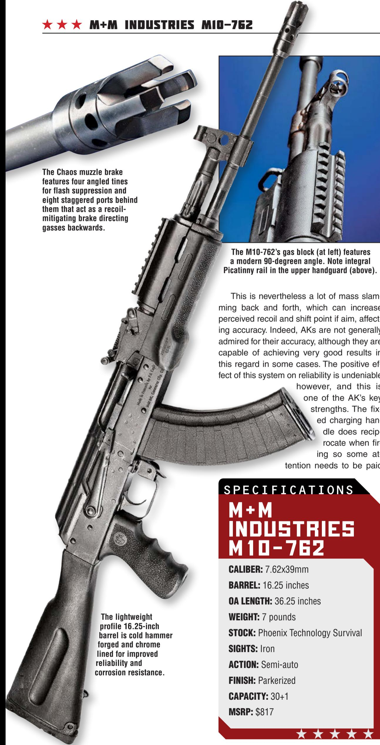
The Chaos muzzle brake features four angled tines for flash suppression and eight staggered ports behind them that act as a recoil-mitigating brake directing gasses backwards.
